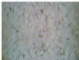
Surface finish of GM circuit at 400x
